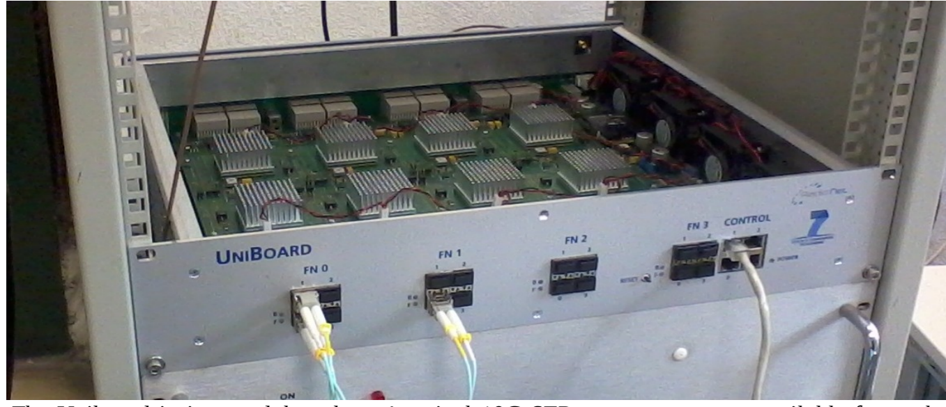
The Uniboard in its standalone box. 4 optical 10G SFP+ connectors are available for each Front Node FPGA, and the board is controlled using standard Ethernet.
