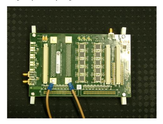
Connect these ground straps to the DBBC housing. Ensure a good contact. In our example the side wall was used. In case of an internal Fila10G this space is occupied. Any other position will do.
