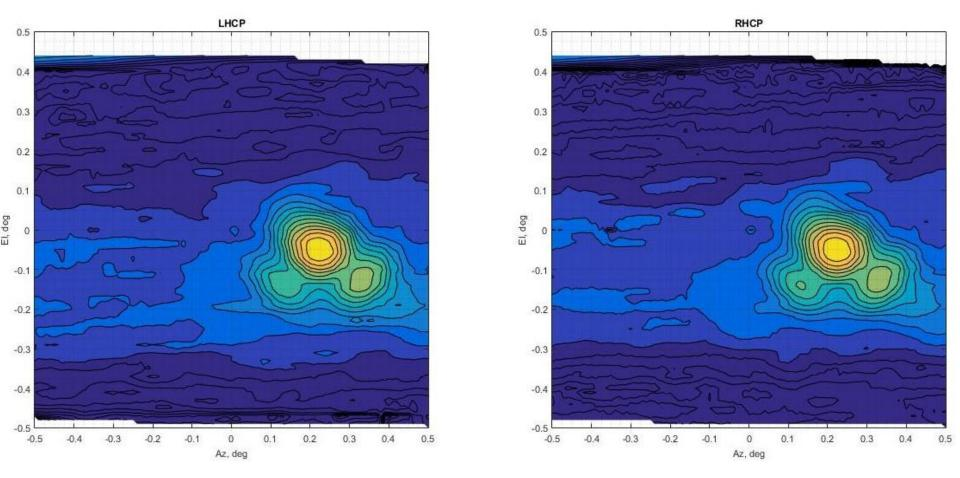
Source Casa; no pointing model; Elevation 30 deg; Freq: 7.6-8.8 GHz; (total power); Countours 1dB; Max 64 dBi. Date 24.08.2016.
