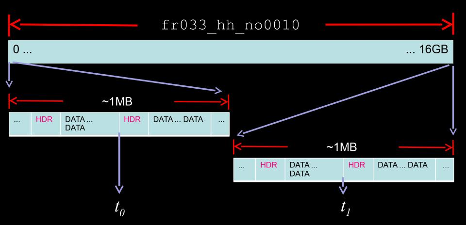
data rate =  $\delta t / \delta bytes = (t_1 - t_0) / recording length$
