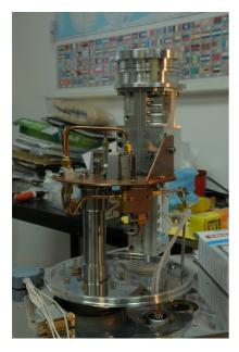
A new C band (4-8 GHz) receiver has been installed on the antenna on May 21 2015. Currently it co-operates with an old methanol band converter. The new wide band converter is almost complete and will replace the substitute soon. The first measurements shows a significant improvement of sensitivity indicating the system equivalent flux density of about 170 Jy ( $T_{\rm sys} \sim 27 {\rm K}$ ).
