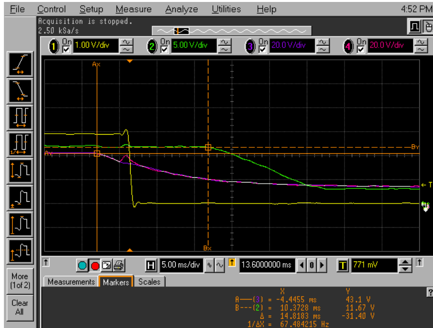
Figure 10 Switch off, showing on/off (yellow), Vcc_12V (green), Vcc_UNB2in (purple), Vcc_brick_in (pink)
