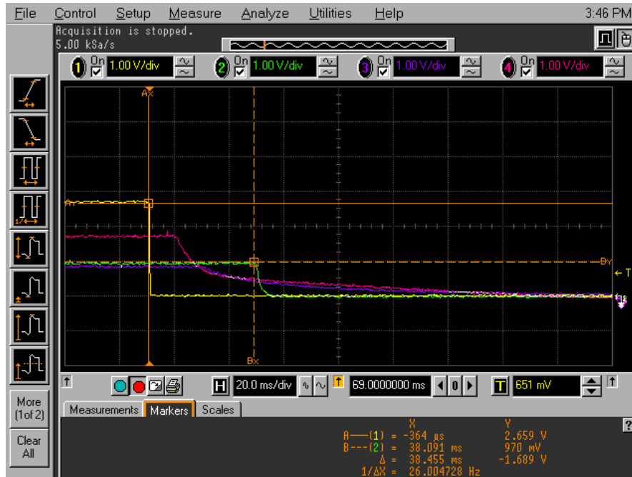
Figure 6 Sequence OFF showing on/off (yellow), Vcc_core (green), Vcc_eram (purple) and Vcc_Bat (pink)
