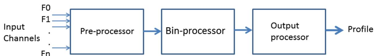
**Figure 1.** Pulsar-binning hardware.
