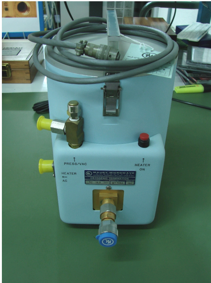
Cold load (model MT7118A Maury Microwave)
