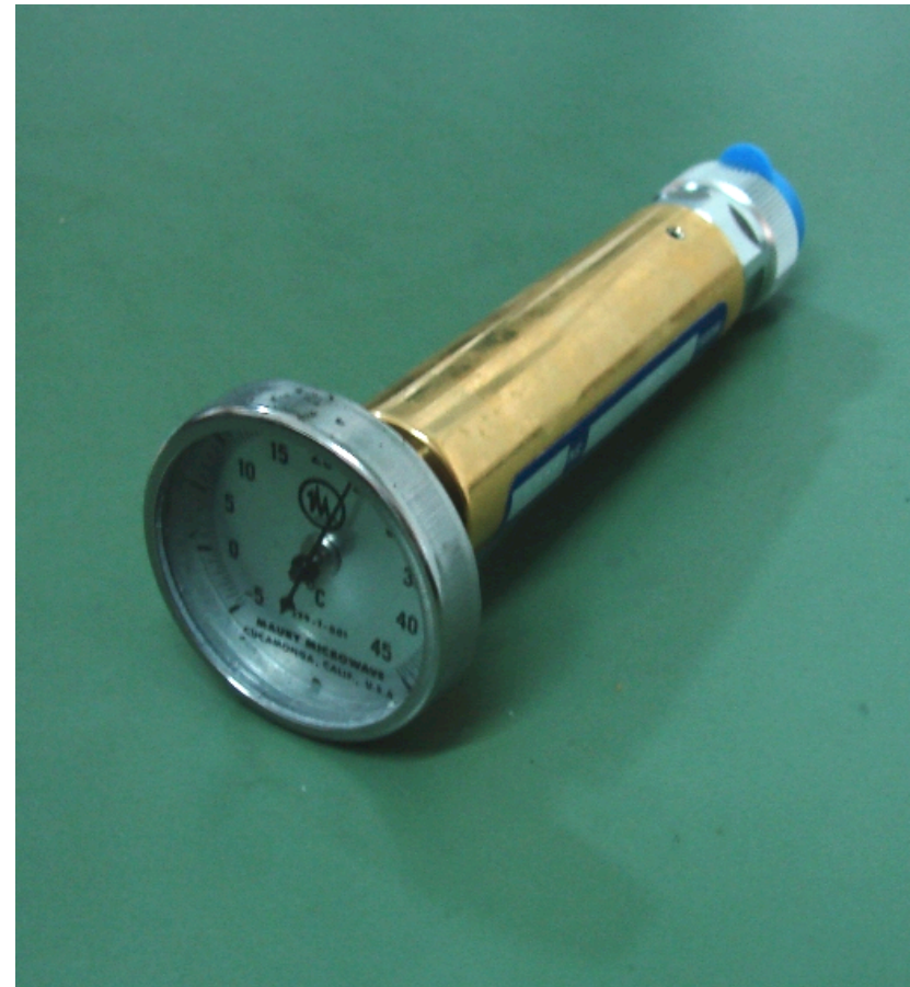
Hot load (model 2695A Maury Microwave)
