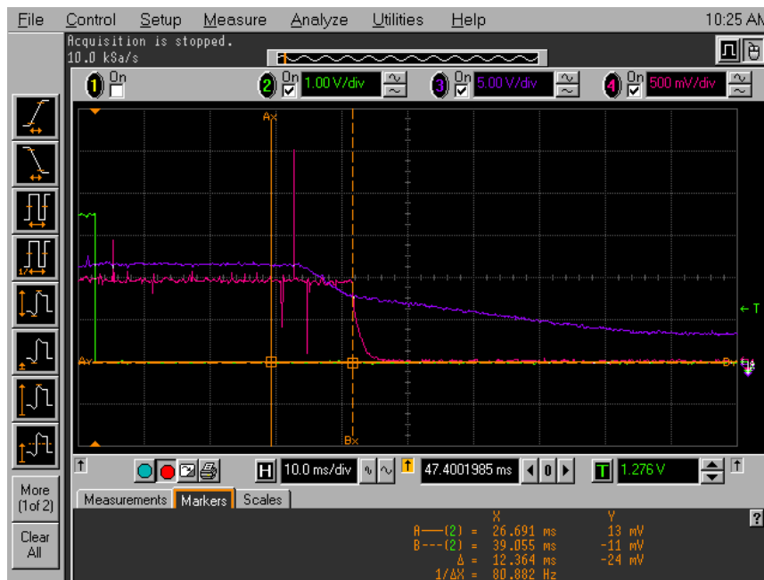
Figure 38 Hold up with 1000uF capacitor.
