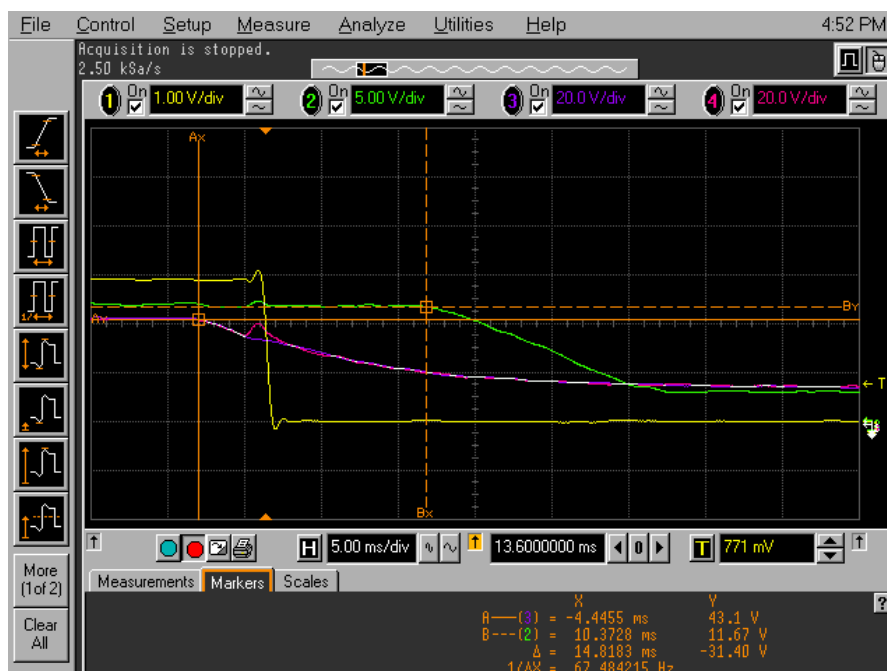
Figure 37 Switch off, showing on/off (yellow), Vcc_12V (green), Vcc_UNB2in (purple), Vcc_brick_in (pink)
