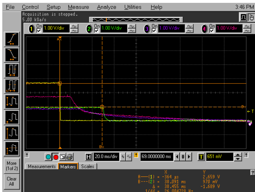
Figure 33 Sequence OFF showing on/off (yellow), Vcc_core (green), Vcc_eram (purple) and Vcc_Bat (pink)
