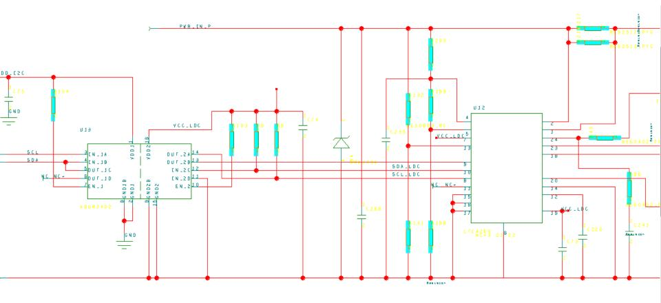
ADIN can be used to measure the input supply ADIN = (1.5/(56.2+1.5) $^{4}$ Vin=0.026 $^{4}$ Vin (Vin=48V-->Adin=1.25V)
