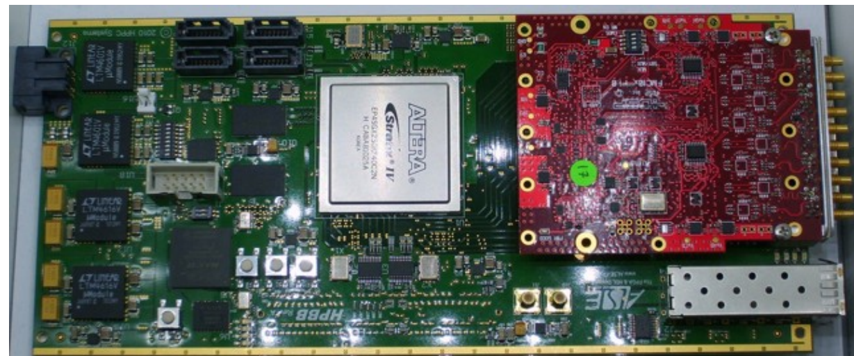
Digital receiver designed and built at Meudon Observatory
